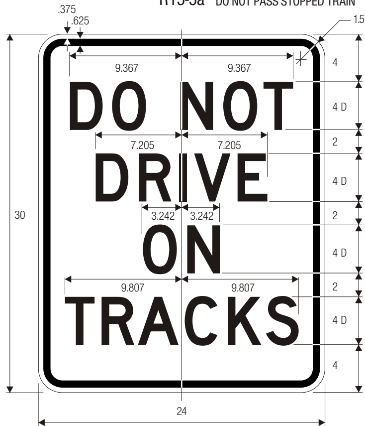
R15-6a DO NOT DRIVE ON TRACKS
